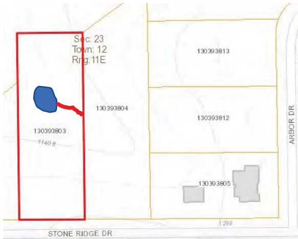
Figure 2 - Drainage area, Rain Garden highlighted in Blue, Dry Creek Bed #1 in Red
