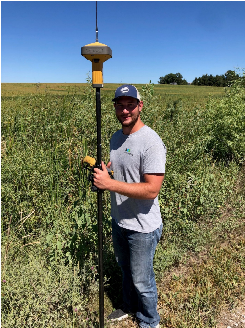
Resources Technician Evan Sisel in the field using Topcon GPS equipment to layout conservation practices
