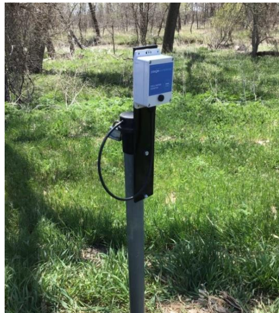
Figure 2 A Paige Wireless device coupled with a pressure transducer on a monitoring well in western Nebraska.
