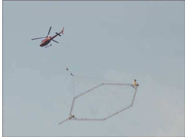
Airborne electromagnetic (AEM) flight over LPSNRD
