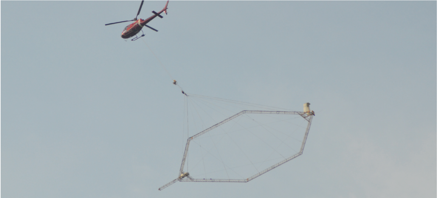
Sensing equipment suspended from a helicopter can detect variations in geological materials and locate possible aquifers several hundred feet below the surface.
