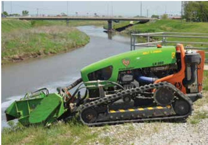
**No Seat/No Problem** - This remote-controlled mower is being used this summer to mow Lincoln's Salt Creek Levee. The NRD is responsible for maintaining the 13-mile levee system and mowing it several times each year makes it easier to inspect drainage structures and easier to monitor the levee during high water events. Using the remote-controlled mower reduces the likelihood of someone being injured mowing the steep slopes.
